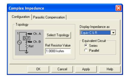
When the 'Select Topology' button is clicked the topology selection dialog is displayed which displays six configurations for Device Under Test (DUT) connections. Choose the topology which matches your setup. The 'Select Topology' and 'Parasitic Compensation' dialogs are shown below.
